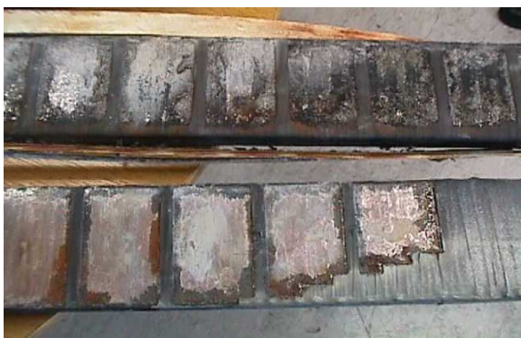
Figure 15. Abrasion of the slot corona protection due to vibration
