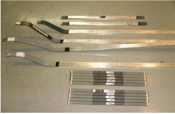
Figure 8. Different types of model bars used for voltage endurance measurements
